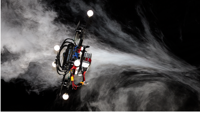
Fig. 2: Our quadrotor platform reaches its physical limits at a pitch angle of 80 degrees while performing a lemniscate trajectory in our experiments. Throughout the trajectory, the platform reaches speeds of up to 14\text{m s}^{-1} and accelerations beyond 4g .
